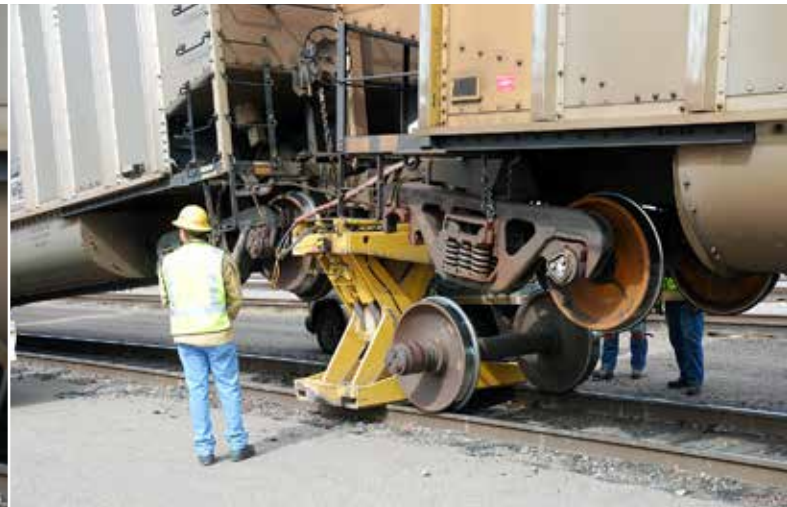
2 As the cars rise, a crewman attaches safety hooks to the wheelset to be changed out to ensure it doesn't roll away as it disengages from the truck's sideframes. Four photos, David Lustig
